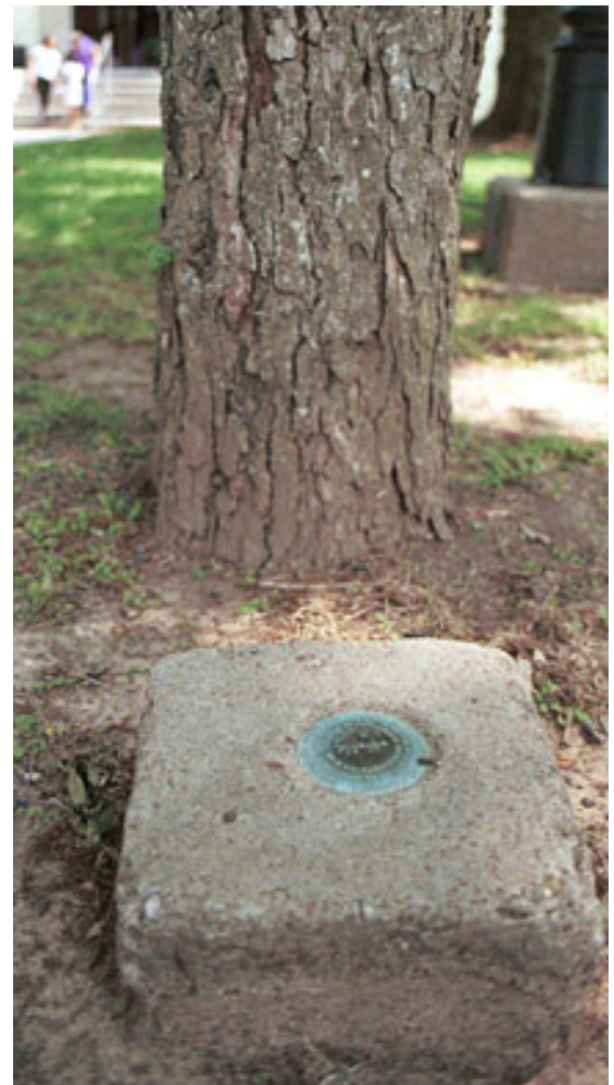
The United States Geological Survey's flood-elevation "reference" marker protrudes from the ground near the county courthouse.
